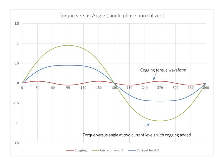
Figure 2 above shows a typical torque versus angle curve for a rotary motor. It is depicting only one of the three phases of the motor. Two levels of current have been selected to show how torque changes with current. Cogging torque at 5% of the rated torque value is shown. Notice how the cogging torque impacts the total torque by reshaping the total torque output, especially at lower current levels.
