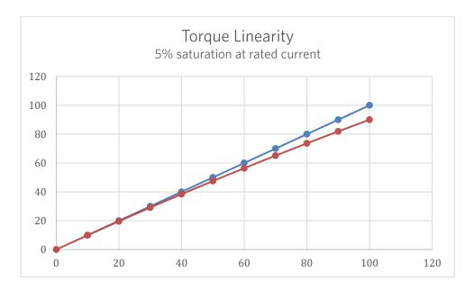
This is more evidence to debunk the theoretical notion that Kt = Ke in brushless permanent magnet motors. Every motor is different, a designer may have optimized Km and weight knowing that there would be saturation.
