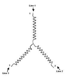
Figure 1 above is a resistor network representing a "wye" configuration. This represents three power input wires and the return of each phase connected together in a center tap inside the motor.
